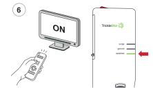
Turn the TV on. Within a few seconds, the switched outlets will have power and the devices plugged into them and can be used.
