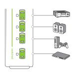
Plug any peripheral electronics, such as a DVD player, receiver and soundbar, into the outlets labeled "switched."
